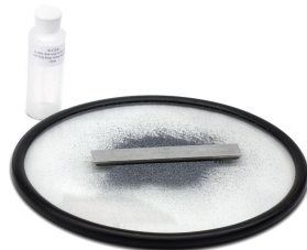
60 GRIT SILICON CARBIDE POWDER OR SANDPAPER ON GLASS
